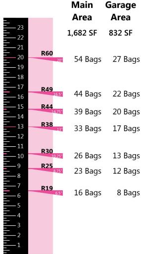
Note: The numbers above reflect the number of bags needed to achieve the specified R-Value. Always subtract the existing attic R-Value from the numbers shown above before ordering material.
